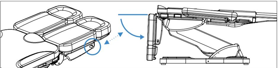
Press the lever to adjust the angle of the legs.
